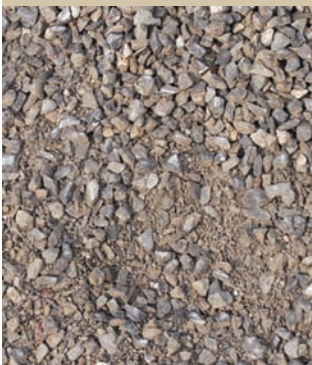
Chippings to Dust
