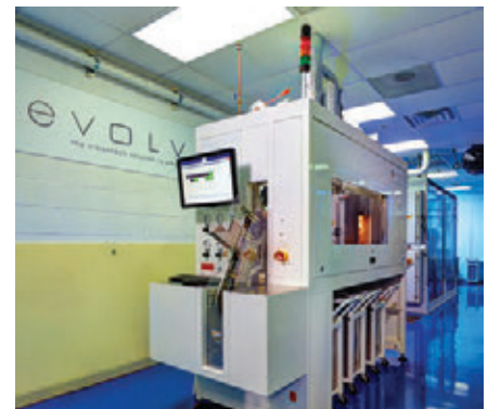
The eVOLV™ Board Clearing Machine (BCM) is used to depopulate components and heat shields from mobile phones.
