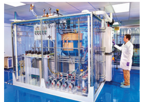
The eVOLV™ Solids Processing Technology (SPT) uses an all chemical, non-grinding, non-shredding process step used to extract precious metals and base metals from integrated circuits.
