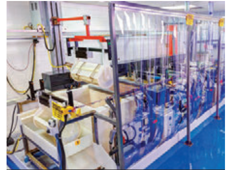
The eVOLV™ process tool contains a series of non-toxic chemistries that extract precious metals and solder metals safely and efficiently from printed wiring boards of all types.
