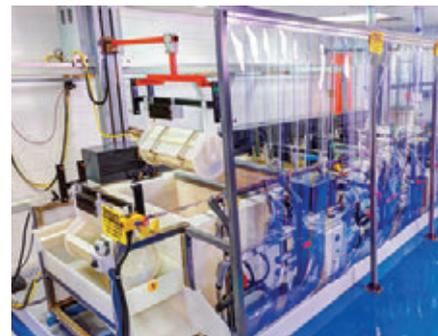
The eVOLV™ process tool contains a series of non-toxic chemistries that extract precious metals and solder metals safely and efficiently from printed wiring boards of all types.
