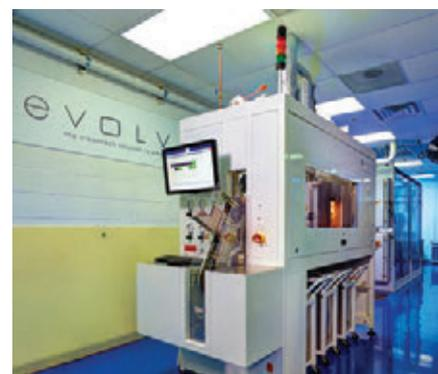
The eVOLV™ Board Clearing Machine (BCM) is used to depopulate components and heat shields from mobile phones.
