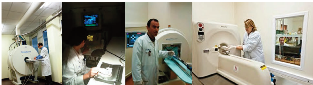
Figure 3. Different types of imaging modalities for preclinical evaluation of nanosystems. From left to right : MRI, Ultrasounds, SPECT, PET (SFR X. Bichat, Paris Diderot-Inserm U1148)
