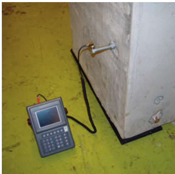
Using an FFT analyser to measure the frequency spectrum of an isolated block
