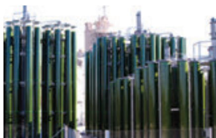
Figure 2. BFS' tested and certified (SGS) Industrial plant that absorbs CO 2 emitted from an adjacent cement factory. Watch a video of the Plant Tour here
