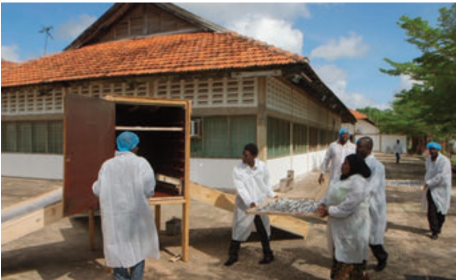
This combined solar smoking and drying unit was designed through collaboration with Matis. It requires far less wood than conventional smoking and drying methods and improves the quality and safety of the product. Demonstration units have been constructed and tested in short courses held in Kenya and Tanzania as seen in this video: http://www.youtube.com/watch?v=WZE64ssYgjY
