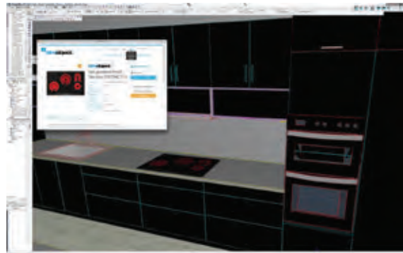
Kitchen layout in a BIM model including a cooker hob object created with BIMobject Mosquito.
