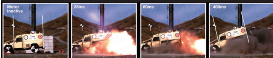
February 2015. Demonstration of ABBS Vehicle Global Acceleration Mitigation system completely eliminating the global acceleration of the vehicle. Vehicle doesn't move at all while the Linear Rocket Motor (LRM) is firing, there is slight spring re-bounce afterwards motor burnout occurs at about 30ms into the sequence. Without the LRM firing the rear of the vehicle is blown about 1m in the air, as shown below
