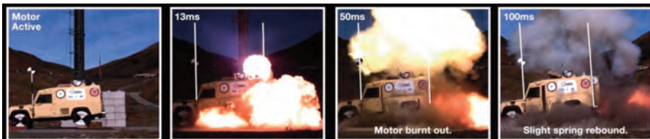
February 2015. Demonstration of ABBS Vehicle Global Acceleration Mitigation system completely eliminating the global acceleration of the vehicle. Vehicle doesn't move at all while the Linear Rocket Motor (LRM) is firing, there is slight spring re-bounce afterwards motor burnout occurs at about 30ms into the sequence. Without the LRM firing the rear of the vehicle is blown about 1m in the air, as shown below
