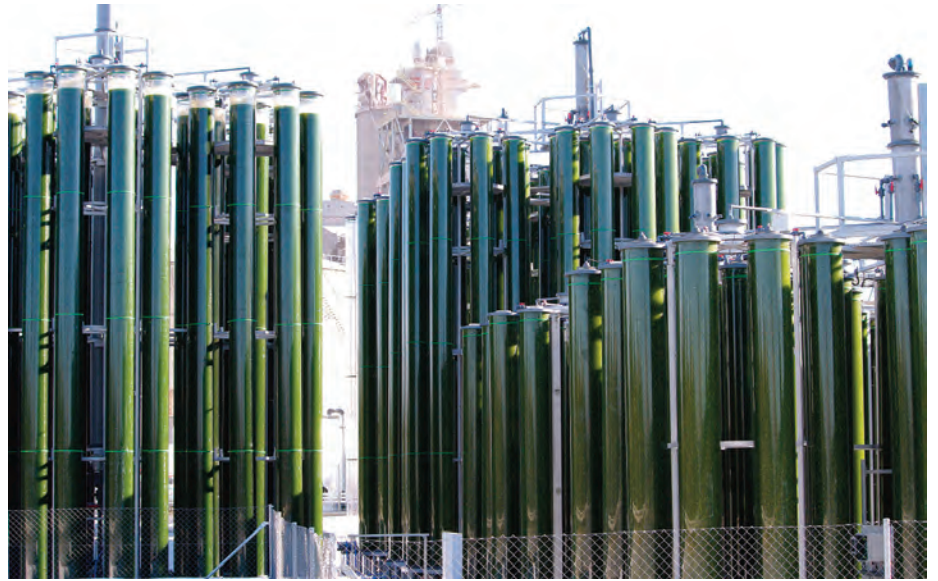
Figure 1. BFS' tested and certified (SGS) Industrial plant that absorbs CO 2 emitted from an adjacent cement factory. Plant Tour: https://www.youtube.com/watch?v=v33kNULlvs
