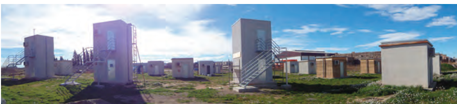
Pilot plant available at the University of Lleida, where TES is tested together with other energy efficiency technologies (good insulation, solar energy, heat pumps, etc.)
