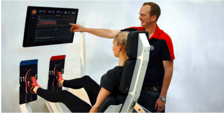
Figure 3: Cardiovascular exercise on a soft robot. A) Soft-robotic device allowing enhanced mechanical loading of exercising muscle in an individual fashion for both legs. B, C) Mechanical characteristics of loading left (blue) and right leg (red) during one work interval (B) and metabolic characteristics (i.e. oxygen saturation) during seven work intervals (C) of interval type exercise on the soft robot.
