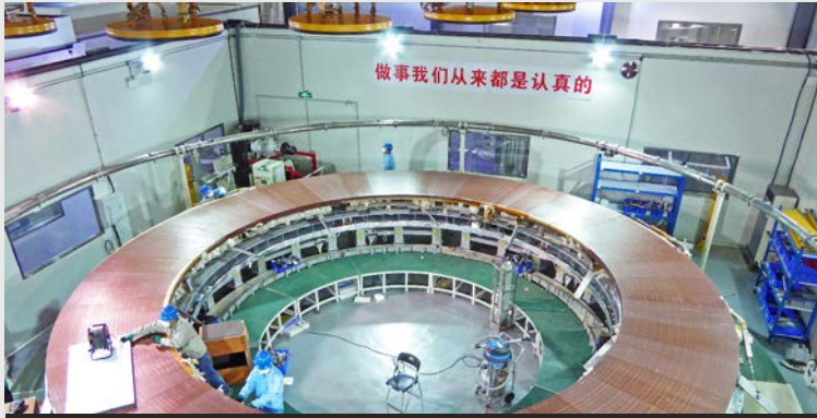
China has completed all of the winding packs for Poloidal Field magnet #6, at the Institute of Plasma Physics of the Chinese Academy of Sciences (ASIPP) manufacturing facilities in Hefei.
