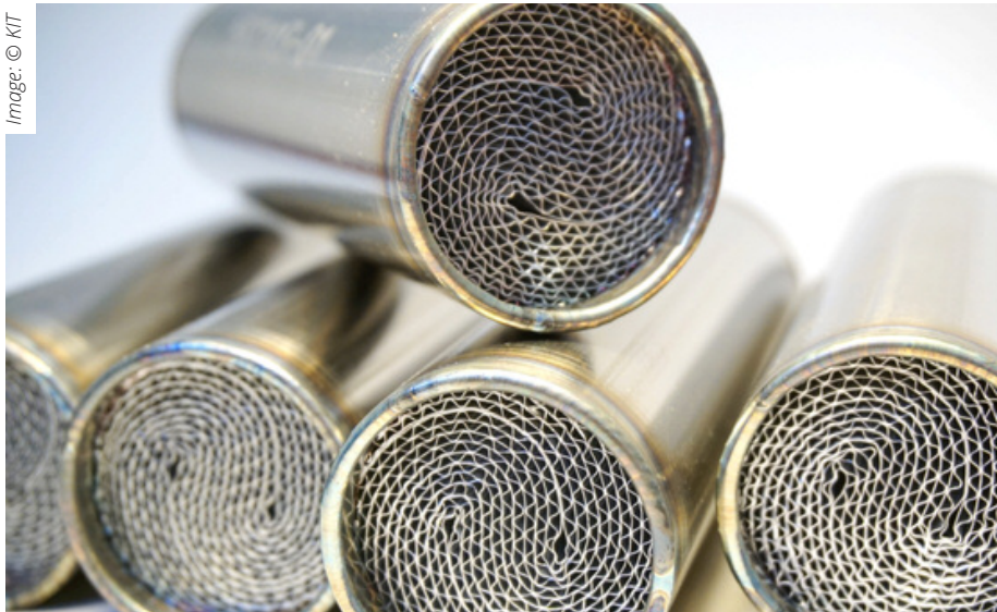
Figure 2: Honeycomb cylinders, the core of the Falkenhagen reactor
