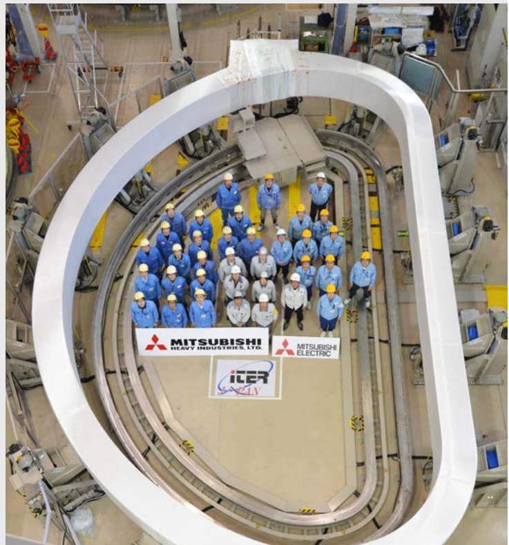
The first toroidal field magnet was completed last year at Mitsubishi Heavy Industries near Kobe, Japan.
