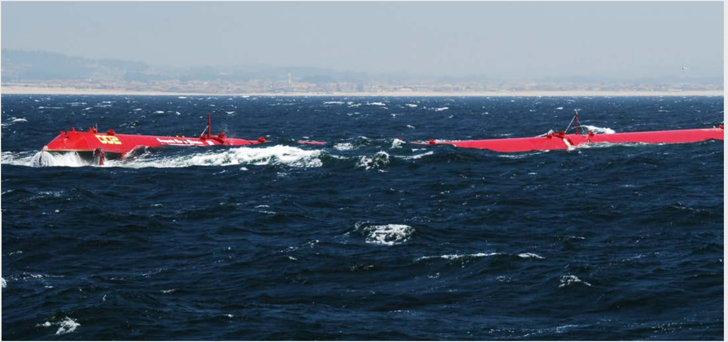
A Pelamis installed at the Aguçadoura Wave Park off Portugal – the world's first wave farm
