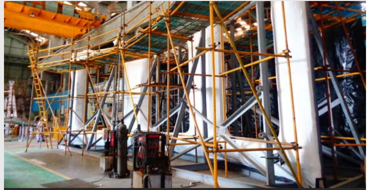
In its heavy engineering facility in Hazira, Indian contractor Larson & Toubro is manufacturing segments of the upper cylinder of the Cryostat: The giant "refrigerator" that will house the ITER Tokamak.
