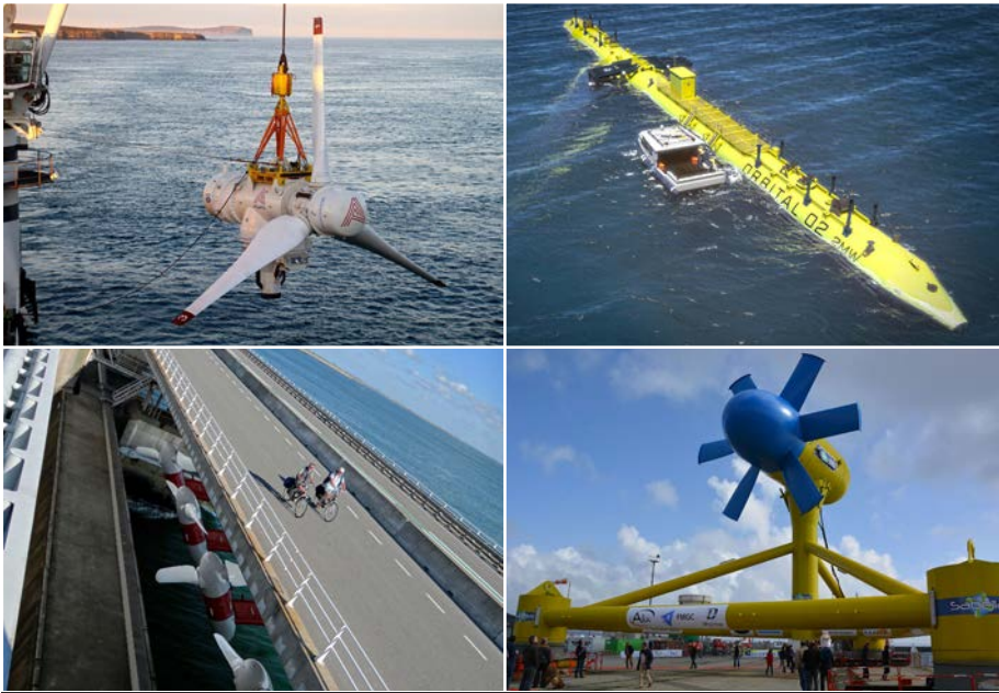
From left to right: Atlantis 1,5MW turbine for MeyGen project, 2MW Orbital Tidal, 1,5MW Tocardo Tidal Power dam-integrated installation, 1MW Sabella turbine for Ushant Island
