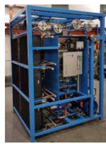
Compressor, turbine, generator unit
