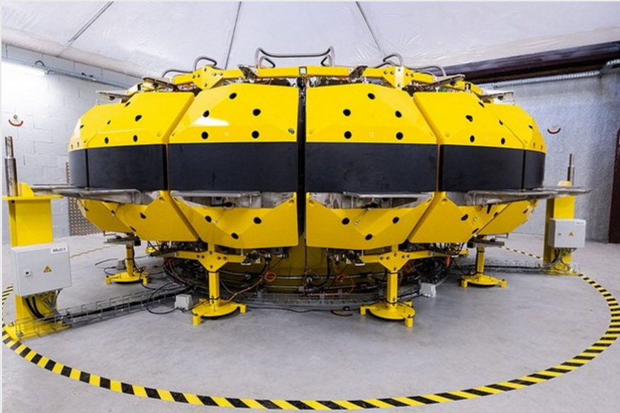
A specialised tool created by Douce Hydro to test the performance of ITER's "pre-compression rings"
