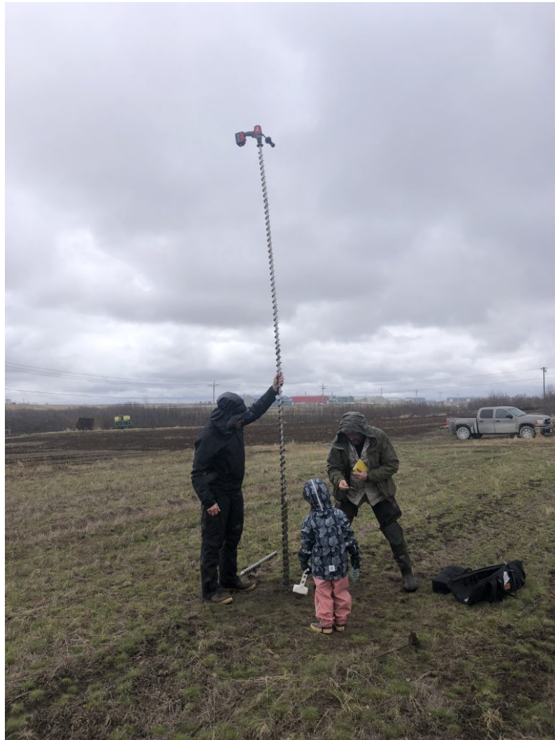
Figure 2: Permafrost Grown team members drill to the permafrost table at a farm in Bethel, AK, using an electric drill with an auger attachment. The image shows ~4 m of auger flights pulled from the ground after permafrost was found.
