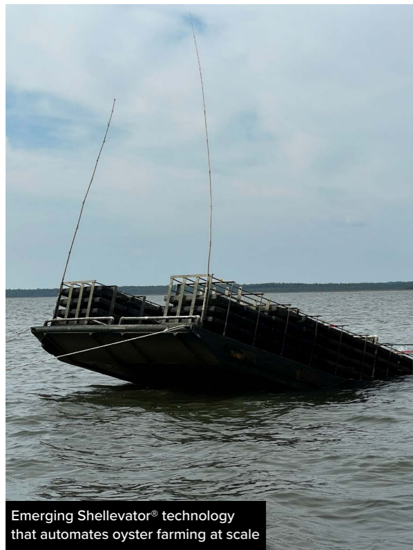
Shellevator® transport of 400,000 oysters to a new area 10km away. The voyage took two hours and used 10L of fuel
